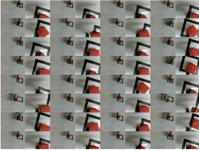
Fig. 2: Samples from the demonstration dataset collected for training the Diffusion Policy. Each frame pair shows synchronized RGB observations from the front-facing and wrist-mounted RealSense cameras during a pushing task.
